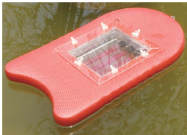
Fig. 3 The kick-board solar reactor in operation in a lily pond at UH (see also Fig. 4). Sample tubes contain Rose Bengal photosensitizer, and the filter is the colorless UVF Plexiglass.
