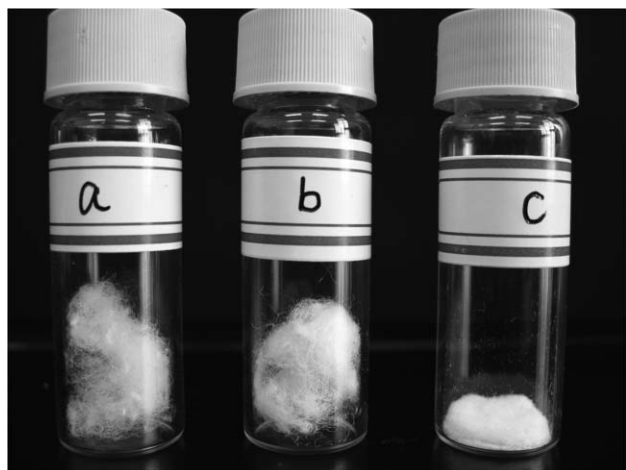
Fig. 1 Photograph of: (a) pristine cotton cellulose, (b) cellulose treated by \text{scCO}_2 and (c) cellulose/ \text{TiO}_2 hybrids prepared in \text{scCO}_2 .
